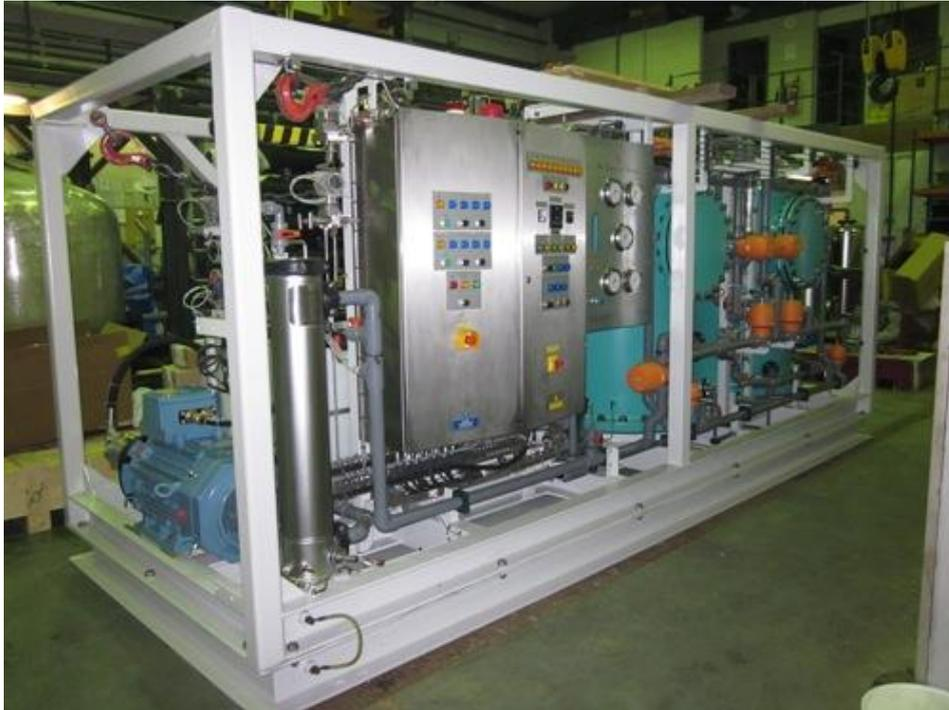
The package was designed, manufactured and tested at our Rochdale works, including all Carbon Steel, Stainless Steel, Duplex and Super Duplex Stainless Steel fabrications.
